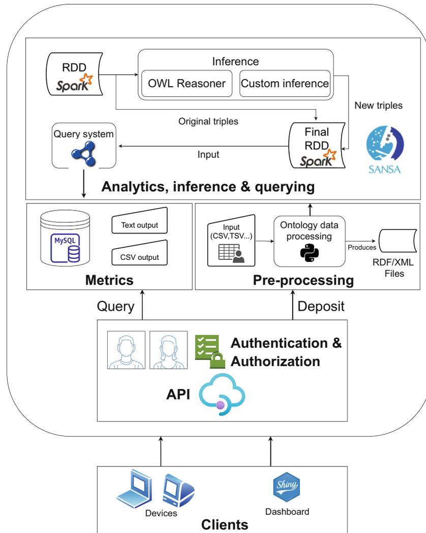
FIGURE 1 Framework's architecture.
